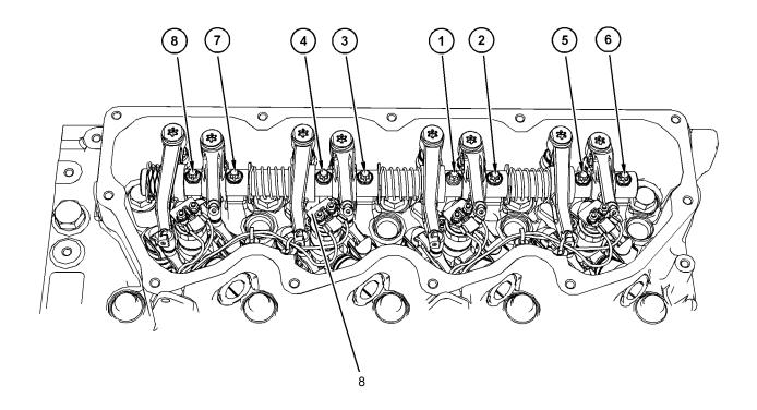
Sequence for tightening the bolts for the rocker shaft assembly
