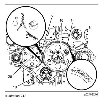
**14.** Ensure that the timing marks on gear (6), gear
