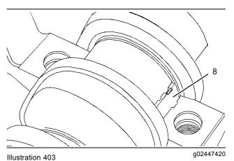
6. Push out upper main bearing shell (8) with a suitable tool from the side opposite the locating tab. Carefully rotate the crankshaft while you push on the bearing shell. Remove upper main bearing shell (8) from the cylinder block. Keep the bearing shells together.
