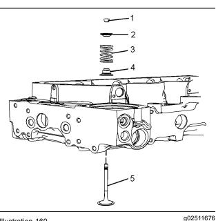
2. Lubricate the stems of valves (5) with clean engine oil. Install valves (5) in the appropriate positions in the cylinder head. Check the depth of the valves below the face of the cylinder head. Refer to System Operation, Testing and Adjusting, "Valve Depth - Inspect" for more information.
