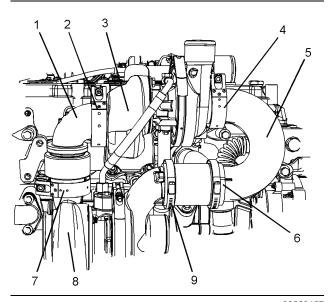
Loosen the bolt on V-band clamp (2) and loosen the bolt on V-band clamp (7) from elbow (1). Remove the V-band clamps from the elbow.
