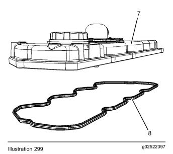
Remove gasket (8) from valve mechanism cover (7).
