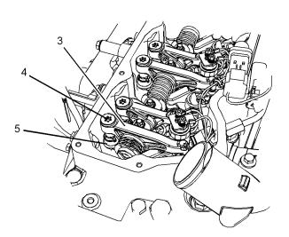
29. Ensure that the guides (5) for the pushrods are correctly positioned on the threaded inserts (4). Use Tooling (E) in order to tighten threaded inserts (4) on all rocker arms (3). Tighten the threaded inserts to a torque of 30 N·m (265 lb in).
