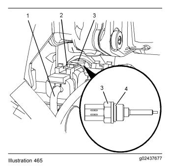
1. Install the new O-ring seal (4) to inlet manifold temperature sensor (3).
