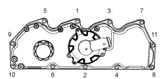
**6.** Tighten the bolts in the numerical sequence that is shown in Illustration 303. Tighten the bolts to a torque of 22 N·m (195 lb in).
