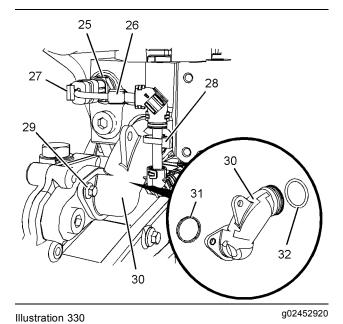
**15.** Use Tooling (C) in order to lubricate the O-ring seals. Install new O-ring seal (31) and O-ring seal (32) to bypass tube (30). Install the bypass tube in the cylinder head. Install bolts (29). Tighten the
