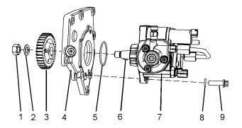
**1.** Use a suitable tool in order to prevent fuel injection pump gear (3) from rotating.
